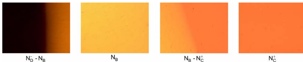
Fig. 3 Lyotropic aligned nematic textures, magnification \times 50 : near the N_D^- - N_B phase transition \rightarrow N_B (20.5 °C) \rightarrow near the N_B - N_C^+ phase transition \rightarrow N_C^+ (22.4 °C). (Online color at www.crt-journal.org )
