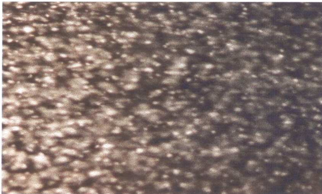
Figura 3.4 Textura da fase L_2 , T = 52,0 \text{ } ^\circ\text{C} ; \text{KL} / \text{DeOH} / \text{H}_2\text{O} ; C = \frac{[\text{KL}]}{[\text{DeOH}]} = 2.90 .
