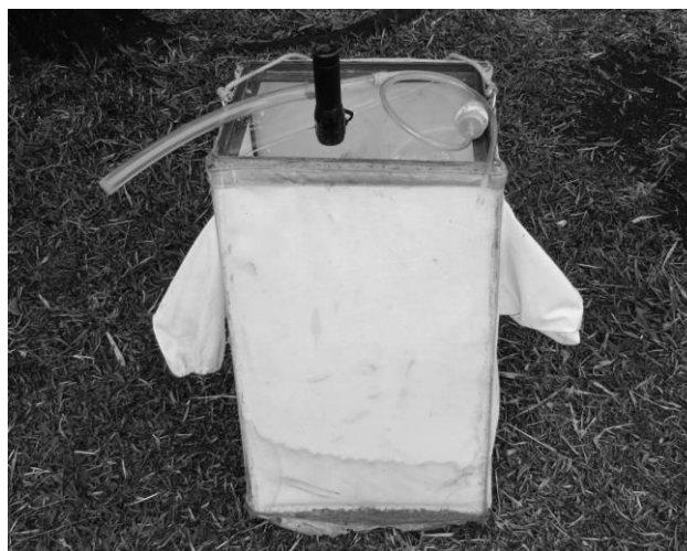
Figure 1 - Quadrangular pyramidal trap (QP), especially developed to collect these insects in wild animal burrows
