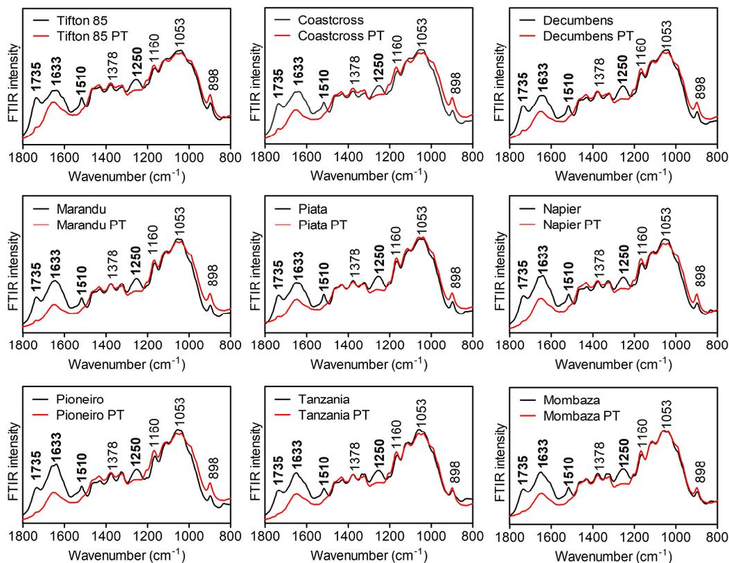
**Figure 4.** FTIR spectra of untreated and NaOH-pretreated (PT) forage grasses. Differences between untreated and pretreated biomasses are presented in bold. Band at 1735  $\text{cm}^{-1}$  corresponds to ester-groups of xylan; 1633, 1600, and 1510  $\text{cm}^{-1}$  correspond to lignin; 1250  $\text{cm}^{-1}$  corresponds to xylan; 1378, 1095, 1060, 1053, and 898  $\text{cm}^{-1}$  correspond to cellulose.
