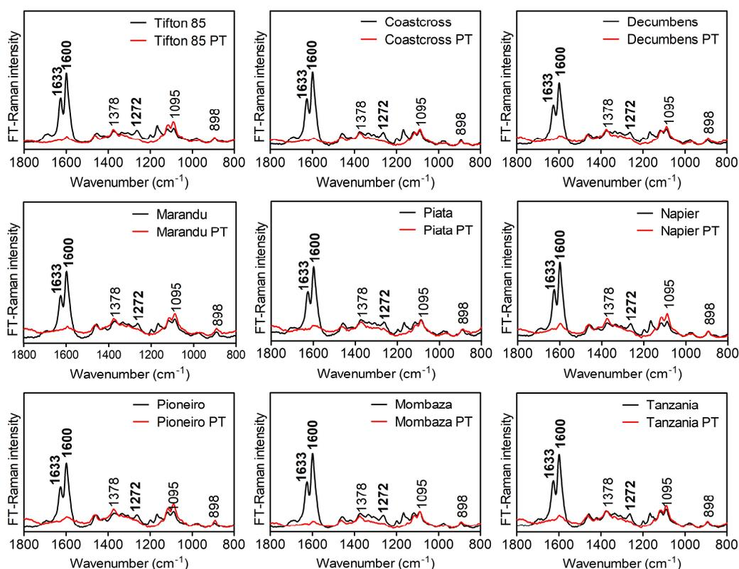
**Figure 5.** Raman spectra of untreated and NaOH-pretreated (PT) forage grasses. Differences between untreated and pretreated biomasses are presented in bold. Bands at 1633, 1600, and 1272 correspond to lignin, 1095 and 898  $\text{cm}^{-1}$  correspond to cellulose.
